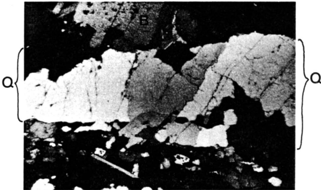
Fig. 3. Photomicrograph of specimen D, taken from the central part of the shear zone; a portion of an elongated lens of quartz grains (strain-free, due to post-tectonic recrystallization), set in a matrix of biotite and oligoclase. Q = quartz, B = biotite. Scale bar 0.5 mm.
